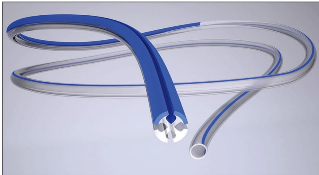
Fig. 2 - A wound drain can be created as a single extrusion with two or more distinct geometric cross-sections and a smooth, integrated transition where the hub had been.
