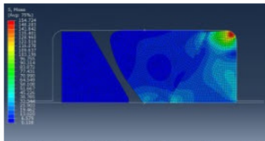
FEA of a Turcon® Wedgpak® from Trelleborg Sealing Solutions
